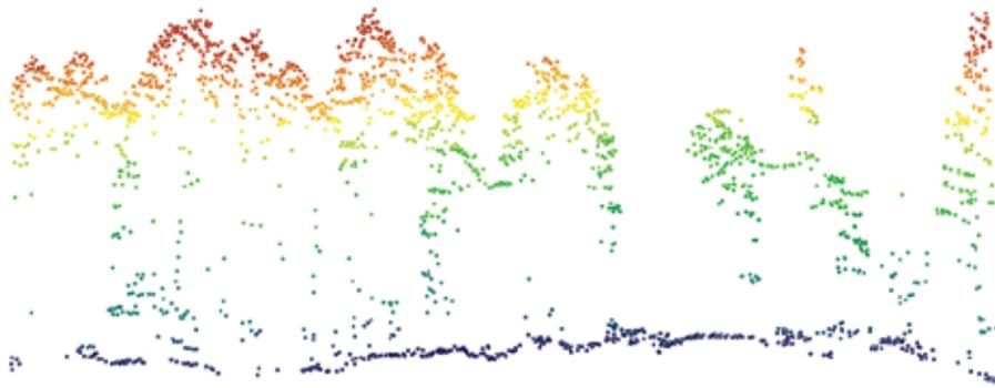
This image shows a cross section of points that are colour coded to indicate their height above ground, illustrating LiDAR's ability to map both the canopy and the ground beneath.
