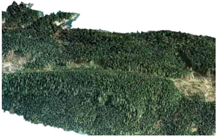
This image is a modified aerial photo draped over a digital surface model. It is an example of how LiDAR data can be combined with other datasets to model stands and also to communicate with stakeholders by means of realistic and detailed 3D visualizations of a particular area.
