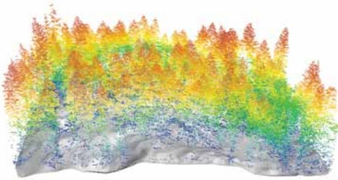
This image is made up of a hillshade image combined with LiDAR points to show a model of forest from top to bottom. LiDAR "point cloud" datasets can be very dense.
